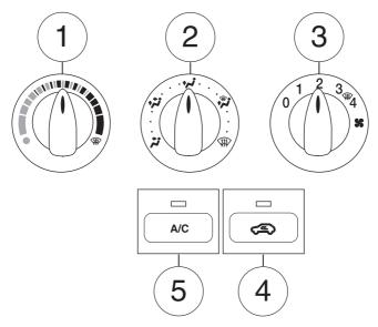
1. **Temperature control:** Controls the temperature of the airflow in the vehicle. For optimum defrosting performance, set the dial to the defrost symbol  $\sqrt{44}$ .
